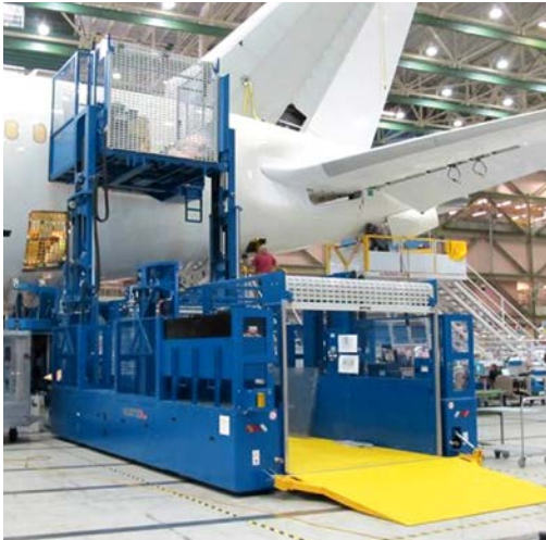
An assembly and work platform with 4-mast lift system
