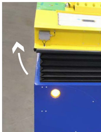
Platform truck for transporting the tail unit in a painting plant with platform lift
