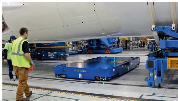
The SL-AGV platform truck transports an aircraft fuselage
