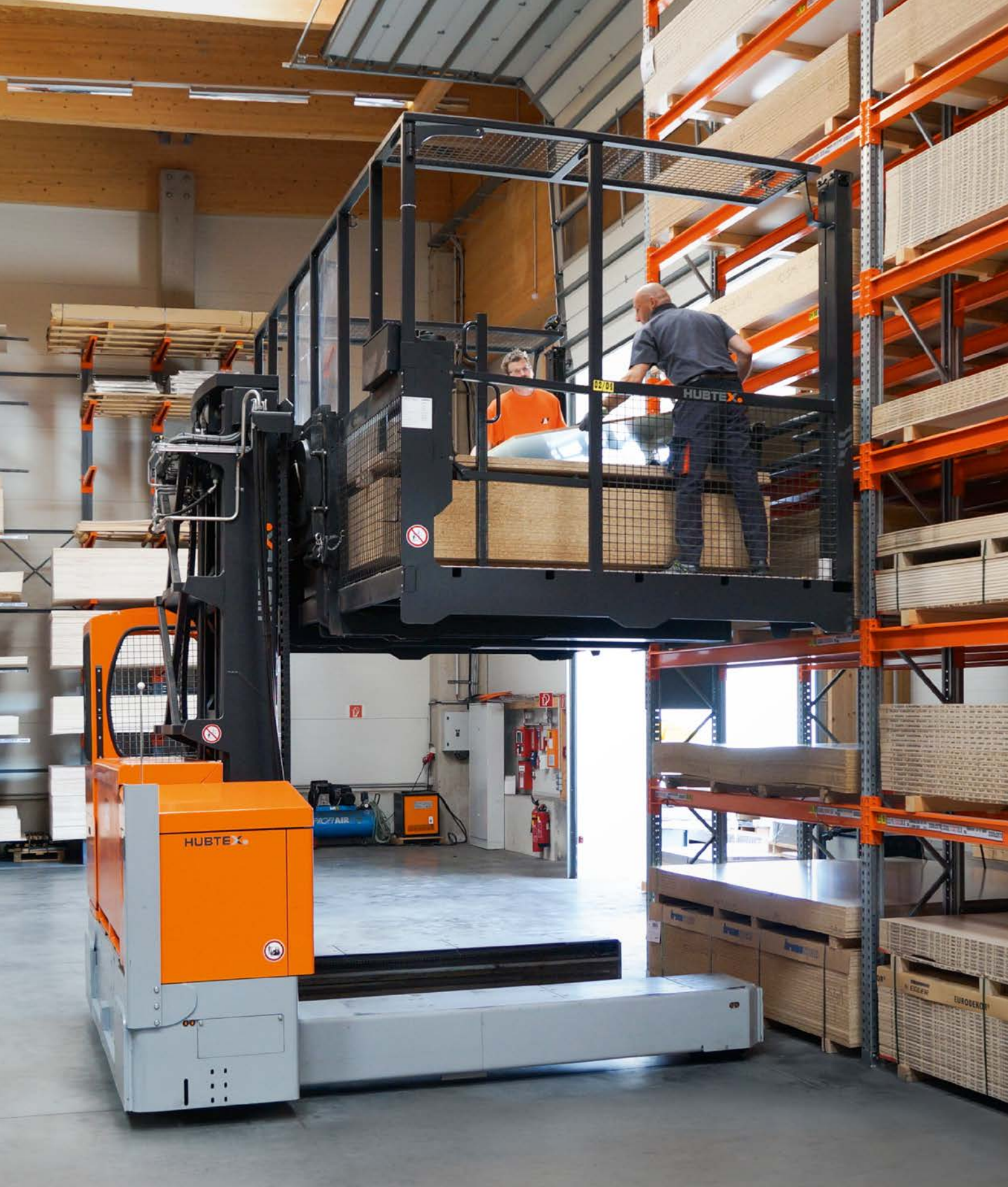
Multidirectional sideloader with detachable order picking platform
