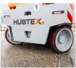
Thanks to a new, patented **single-wheel steering system**, the turning radius is also significantly reduced. The reduction is around 50% compared to the standard steering system. In this case, the pivot point of the vehicle is ideally in the centre of the drive axle.
