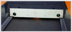
sensors for automatic speed reduction during stillage pick-up
