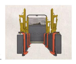
GTR with 180° foldable lifting arms to handle stillages with different widths
