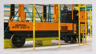
liftable operator's platform for best visibility during stillage handling
