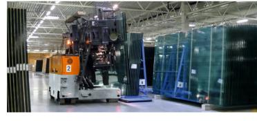
M 150 is able to load/unload a stillage with 30 t glass in 2 working cycles
