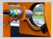
> sensors on clamps to avoid pressure on glass packs
