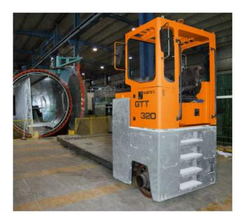
TT loading an autoclave
