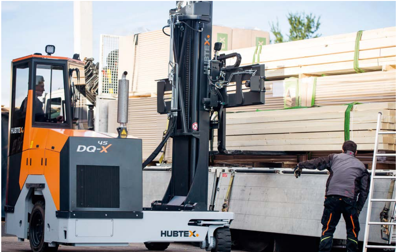
The innovative Stabilisation Assistant prevents undesirable swinging movements during heavy braking.
