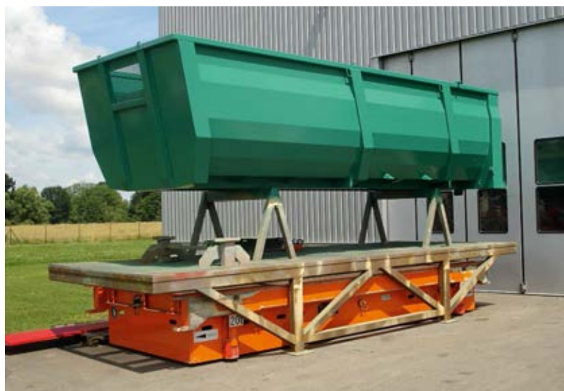
Platform trailer for transporting 65.0 tonnes of heavy tools even on asphalt.
