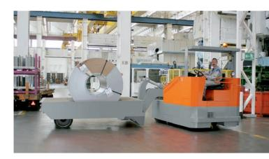
The HUBTEX driver seated Electric towing tractor with swanneck is suitable for handling cargo trailers when coils are to be transported frequently, quickly and reliably.
