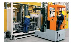
The HUBTEX Forklift Reach Truck model SQ features a combination of compact design and high load carrying capacities of up to 6 t.
