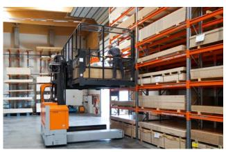
The classic electric multidirectional sideloader in its basic configuration is designed for handling long loads in narrow aisles.
