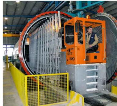
TT unloading an autoclave
