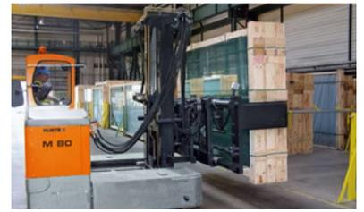
*Multidirectional Sideloaders handles PV-modules on an A-stillage*
