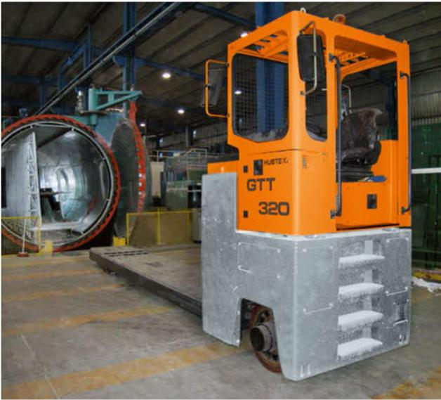
TT loading an autoclave
