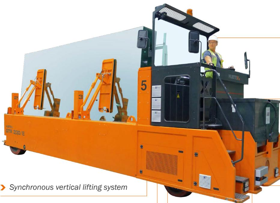
➤ Synchronous vertical lifting system
