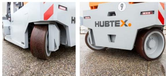
Thanks to a new, patented **single-wheel steering system**, the turning radius is also significantly reduced. The reduction is around 50% compared to the standard steering system. In this case, the pivot point of the vehicle is ideally in the centre of the drive axle.
