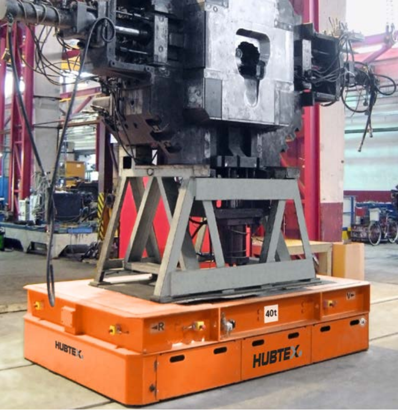
Platform aracı, tařıma kapasitesi 10 – 63 t Platform truck, capacities from 10 – 63 t
