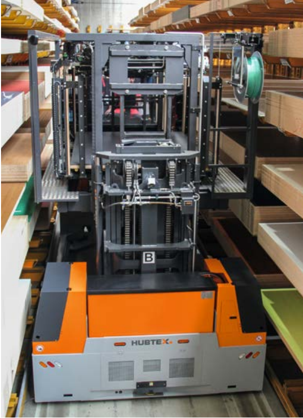
Plaka sipariř toplama iřleminde VacumaX VacumaX for order-picking of plates
