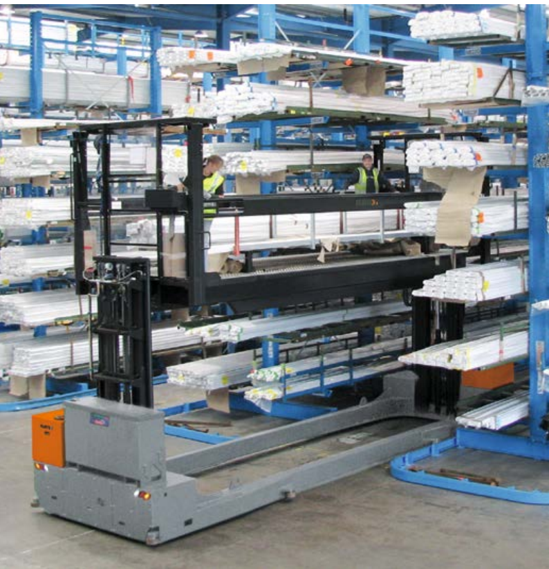
Dar koridorda çift taraflı sipariş toplama Two-side order picker for narrow aisle applications
