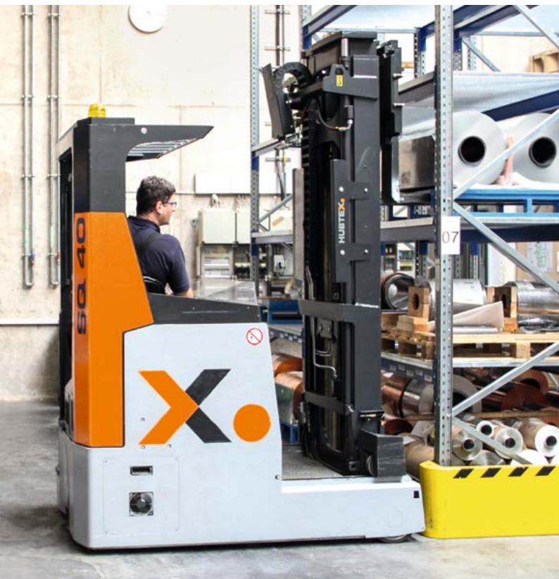
Schubmaststapler in kompakter Ausführung Reach truck with compact design
